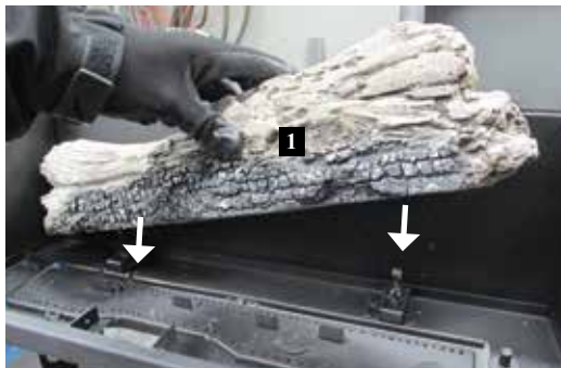
Logs 1 - fits over pins behind burner
